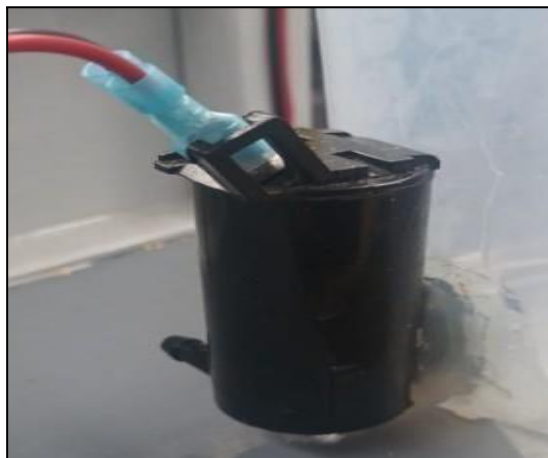
Figure 21: 2-piece 12-volt DC water pump
